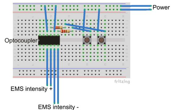
Figure 3: Fritzing diagram of the hacked EMS circuit.
