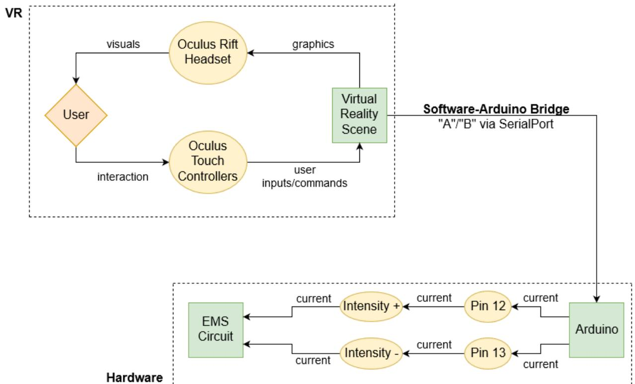
Figure 1: Three part system diagram: virtual reality, software-Arduino bridge, hardware.
